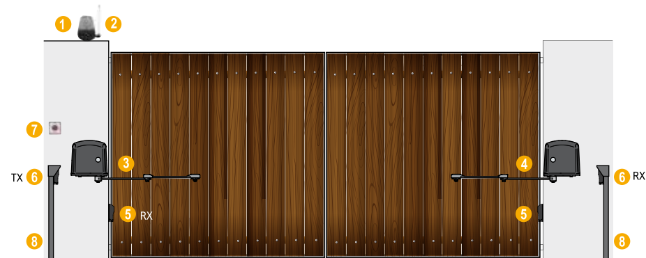
1_Flashing light 2_Outstanding antenna 3_LH operator featuring control board and radio receiver 4_RH operator Motoriduttore destro 5_Outer photocell 6_Inner photocell 7_Key switch 8_Phocell posts
