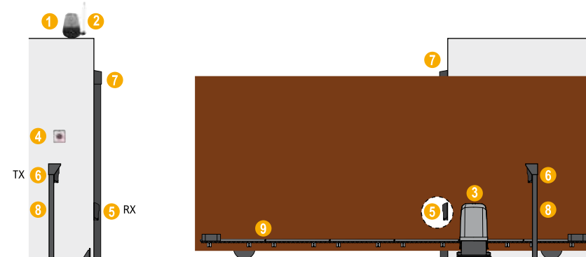
1_Flashing light 2_Outstanding antenna 3_Gear motor complete with control board and radio receiver 4_Key switch 5_Outer photocell 6_Inner photocell 7_Safety strip 8_Photocell posts 9_Rack
