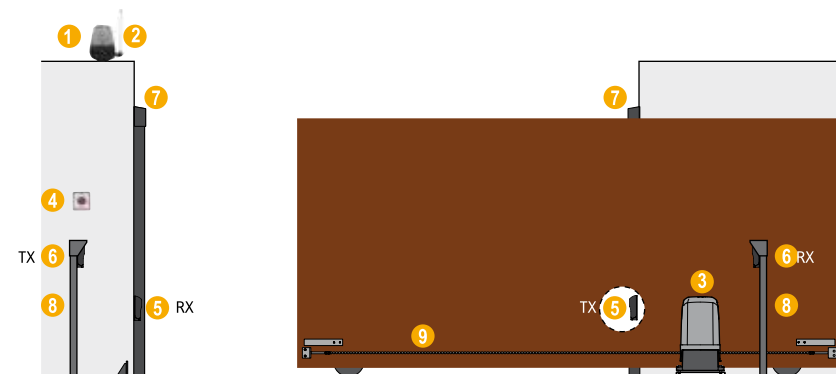
1_Flashing light 2_Outstanding antenna 3_Gear motor complete with control board and radio receiver 4_Key switch 5_Outer photocell 6_Inner photocell 7_Safety strip 8_Photocell posts 9_Chain
